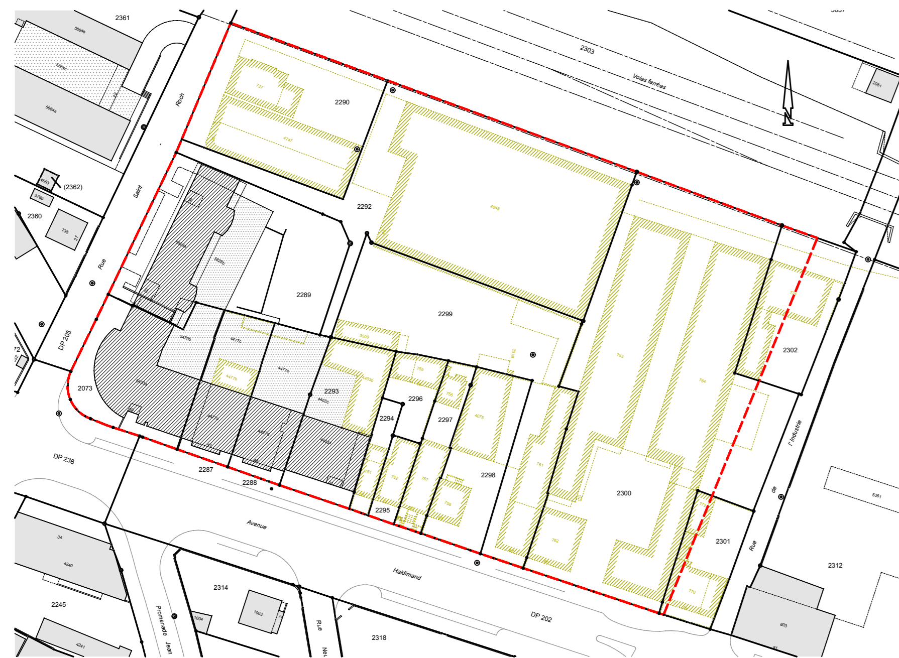
CONSTRUCTIONS CONSERVEES / CONSTRUCTIONS A DEMOLIR - PLAN ECH. 1/1000
